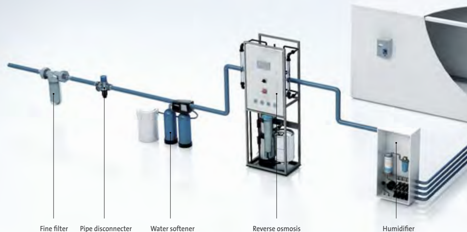
Schematic diagram of a water treatment system for adiabatic humidification
